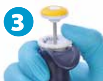
3 Push the thumbwheel down to lock it and start pipetting!
