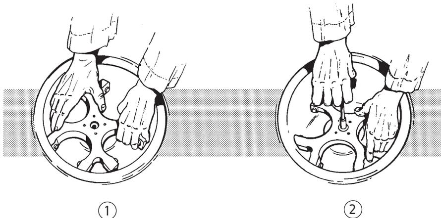
1. Lower the yoke onto the drive shaft
